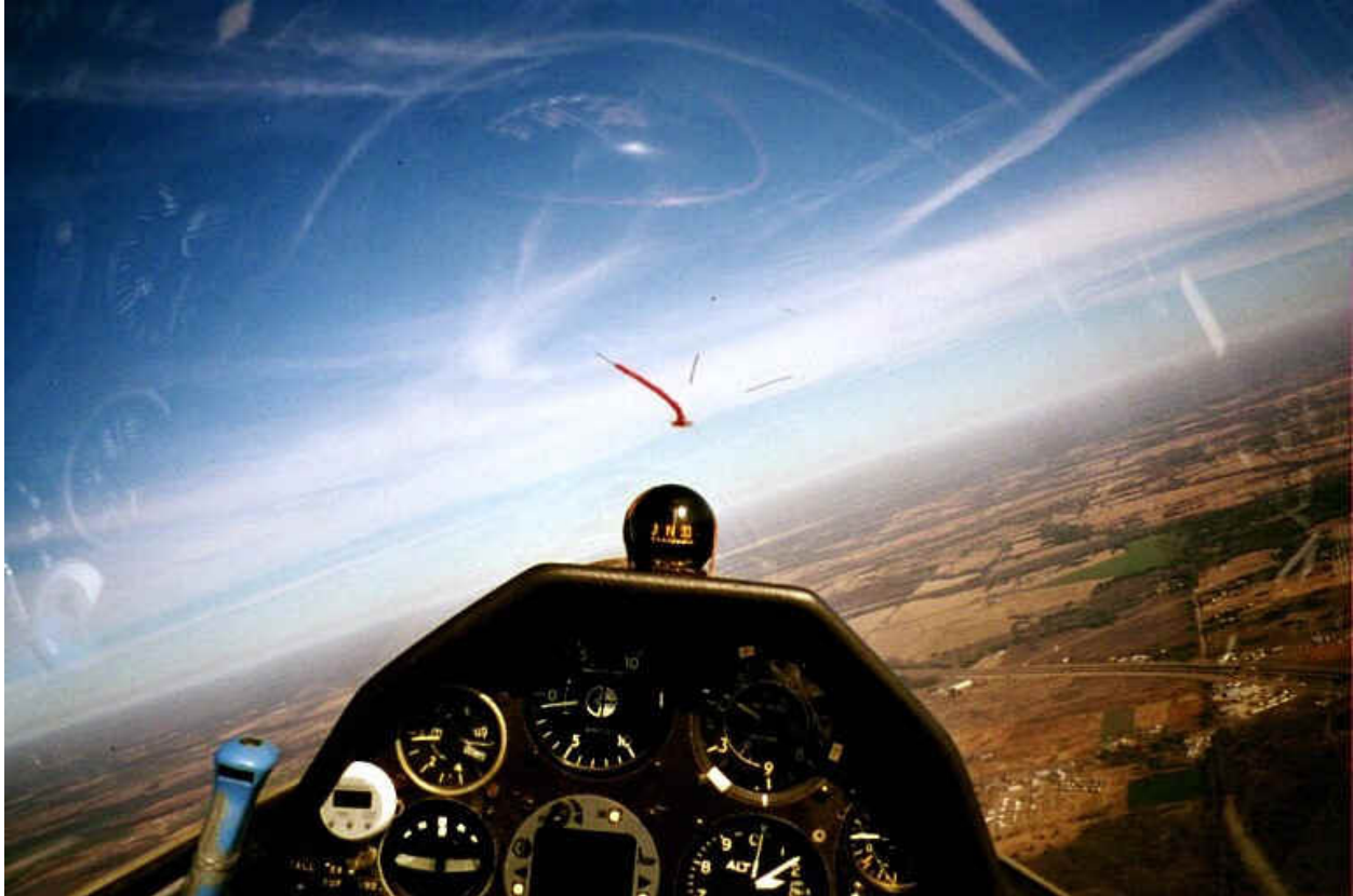
Ventus A instrument panel and canopy view during a gentle right turn. Skid ball is at advocated \frac{1}{2} ball width on the low side of center. Unfortunately, the electric turn indicator is un-powered.
