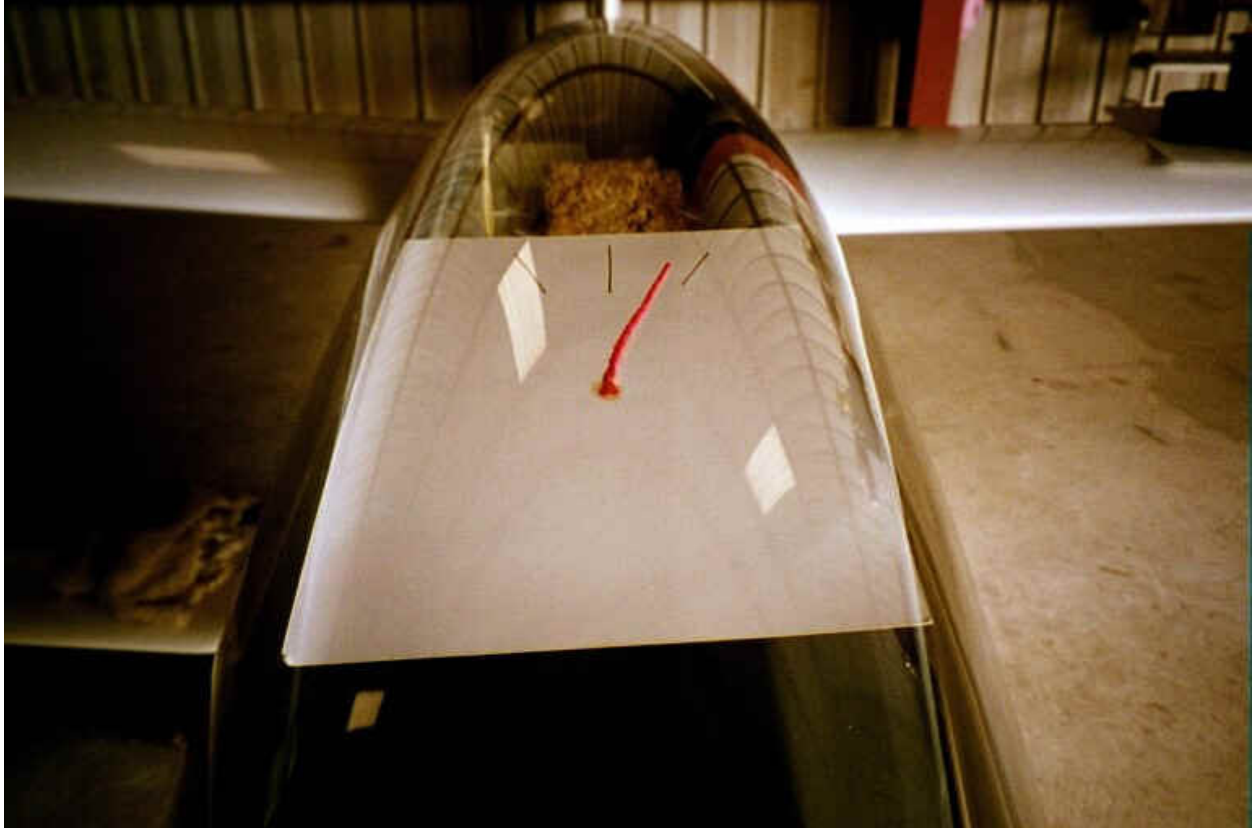
Red yaw string mounted on forward centerline of Ventus A canopy, with \pm 20 degree yaw lines marked in black ink.
