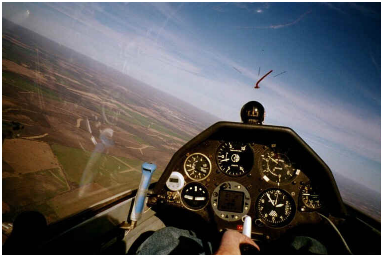
Author's Ventus A cockpit view during a properly coordinated left turn, with yaw string kept about 10 degrees on the high side during the turn.
